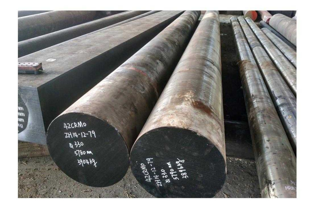
Alloy steels are essentially plain-carbon steels to which small percentages of alloying elements such as chromium and vanadium have been added. The effect of these additional elements is to modify considerably the steels' properties and to make them more suitable for specific applications than are the plain-carbon steels.
